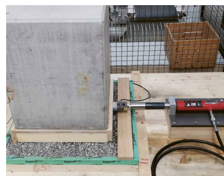
Laboratory test to determine friction coefficients
