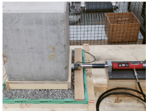
Figure 6. Experimental test set-up for the friction test on a laboratory scale. Source: [10]
